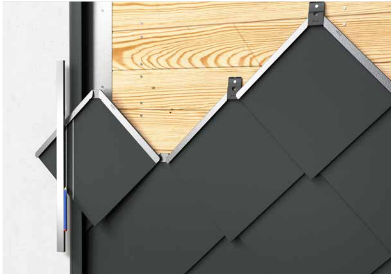
Figure 70 • Raccordement latéral - rebord
